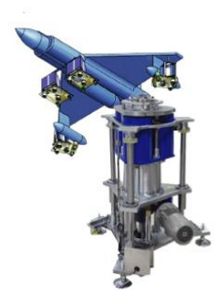
Ground Vibrati on Test machin e
