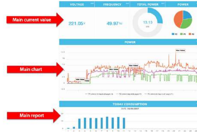
Report workshop energy consumption
