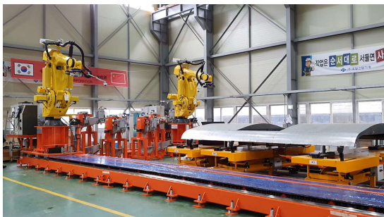
ROOF welding system
