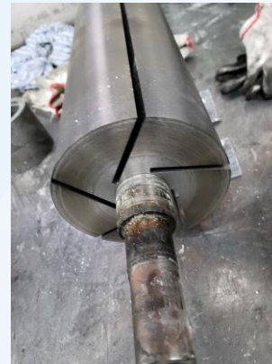
Damage of the entire motor due to bearing faults
