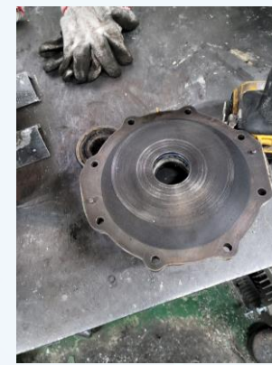
Damage of the entire motor due to bearing faults
